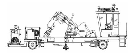
**Air System:** Air compressor is engine oil lubricated, water cooled. System pressure is 100 psi. 613 cu. in. capacity air tank. Service brakes are controlled by a pressure reducing valve and the parking brakes by a manually operated dump valve.
