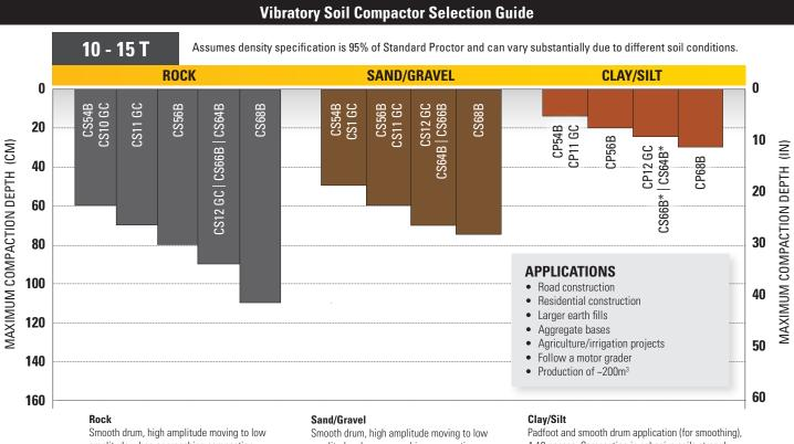
amplitude when approaching compaction, 4-8 passes
