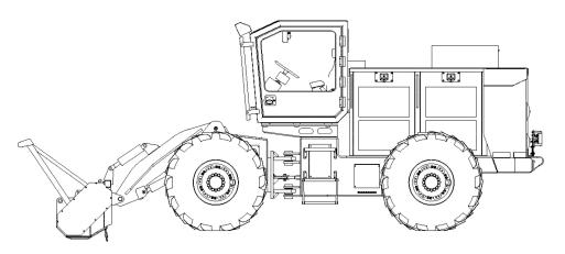
Capacities: Fuel tank: 81 gallons (306.61). Hydraulic tank: 70 gallons (2651).
