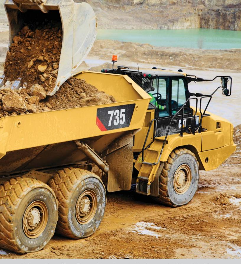
The Cat 735 with a 20  $m^3$  (26.2  $yd^3$ )/32 tonnes (35.3 tons) capacity, offers demonstrated reliability and durability, high performance and productivity and a new world-class cab to improve operator comfort and ease of operation.
