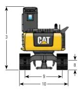
548 LL Log Loader - Under/Under (1.22 m (48 in) riser side entry cab, boom stretched out away from machine)
