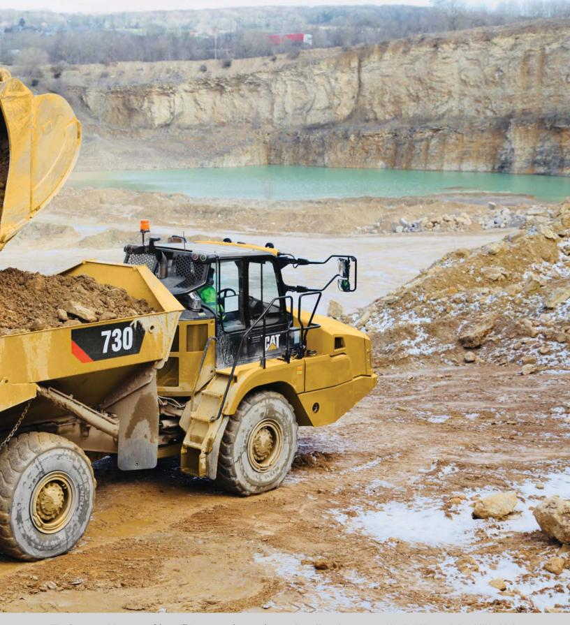
The Cat 730 with a 17.5  $m^3$  (23  $yd^3$ )/28 tonnes (31 tons) capacity, offers demonstrated reliability and durability, high performance and productivity and a new world-class cab to improve operator comfort and ease of operation.
