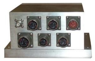
The Intelligent Control Module (ICM) is a flexible central intelligence unit for the collection and interpretation of railway wayside sensors and equipment. Designed to operate in the harshest environments in the world, the ICM is designed as a ruggedized low-power solution for mining and freight applications.
