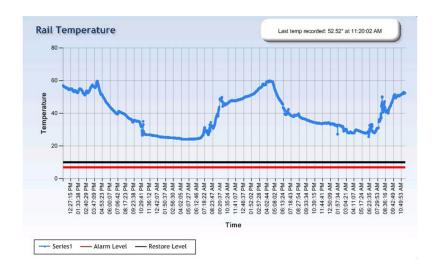
The expansion and contraction of a train system's rails can create great stress on joints and within the steel material. Progress Rail's Rail Temperature Monitor provides continuous temperature monitoring, allowing adjustments to be made to loads and the speed of travel, reducing external stresses and the likelihood of the rail suffering stress breaks.
