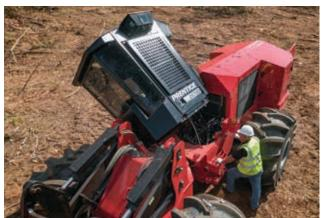
The D Series provides market leading ground-level access to daily service checks, preventive maintenance and emergency repairs.
