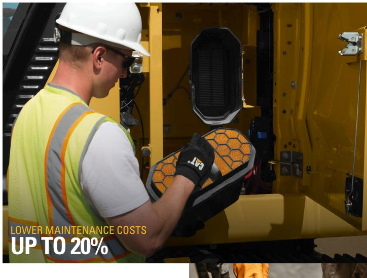
With extended and more synchronized maintenance intervals, you get more done at a lower cost compared to the 320D2 GC. Consolidated filter locations make service faster. Hydraulic, air, and fuel tank filters have increased capacity and longer life.
