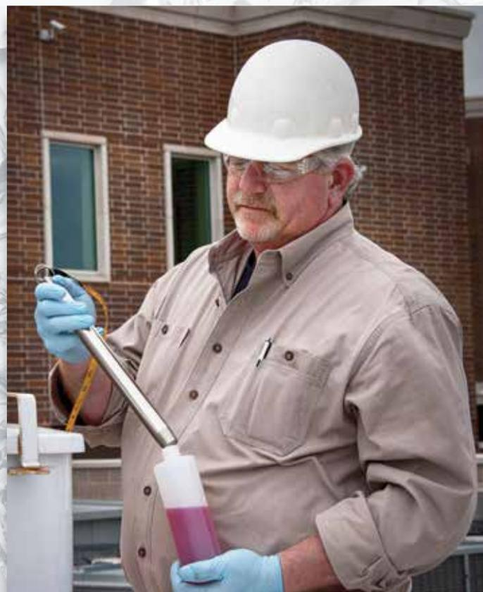
Cooling system testing is often overlooked, but the damage that could occur from overheating won't be overlooked or forgotten. Coolant testing is an easy check to determine whether your coolant has the right chemical balance for maximum system protection and cooling efficiency. We offer two levels of testing for coolant. The first level checks routine characteristics, whereas the second level check provides more in-depth analysis.
