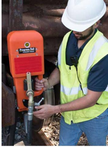
Weighing less than 17 pounds, the End of Train installs quickly and easily with the patented rapid coupler mount design.
