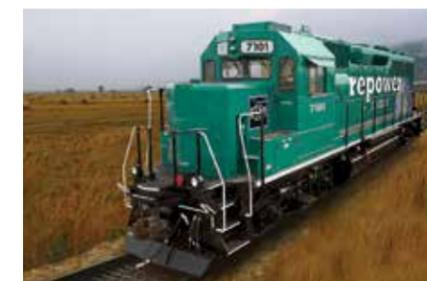
710ECO™ Repowers extend locomotive life for up to 40 years and lower life cycle costs by equipping older models with EMD 710 engines. Benefits include lower emissions, 10 to 25% increase in fuel efficiency, 50% reduction in oil consumption, increased reliability, improved maintainability and enhanced diagnostics.
