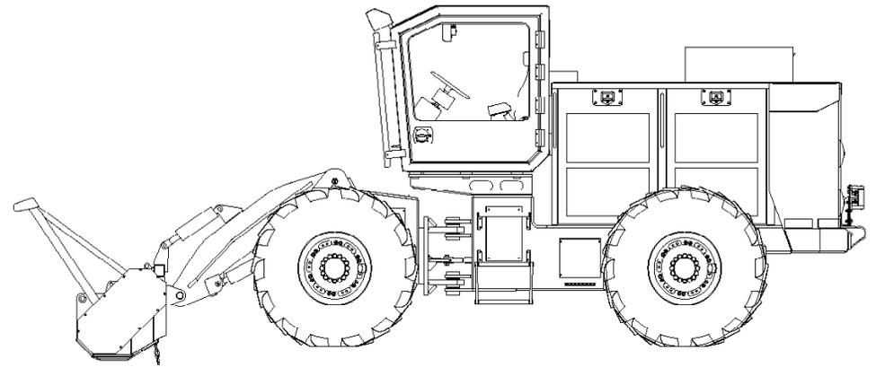
**Cutterheads:** Twin disk rotary cutterhead cuts an 8' swath. Twin disk allows independent rotational control of each disk, allowing better control of debris discharge. Twin disk with rotary axe-type blades cuts up to 8" diameter trees. Shredder cutterhead cuts 7' 1" swath and reduces all vegetation material to a fine mulch.
