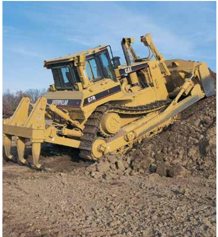
Added track tension increases both the load and the wear on all mating components of your undercarriage. Improperly adjusted track can result in problems and wear on other components:
