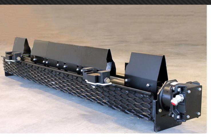
Protect your rolling stock, cargo, concrete ties and track structures from dragging equipment under a moving train with dragging detection technology from Progress Rail Services.
