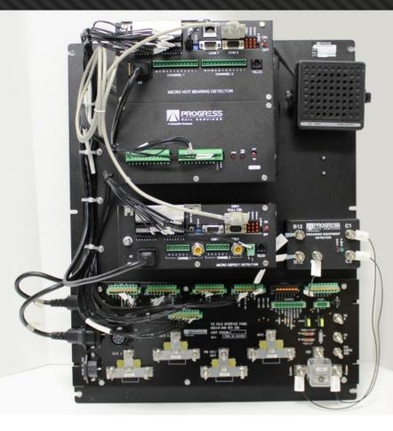
The MicroHBD easily installs in both new and retrofit locations. Upgrade kits are available for various detector systems including Servo 9000s, Servo Cyberscans, Harmon Model 75s, DevTronics CMA02s, and other systems that use Servo ACS I/ ACS II scanners. These upgrade kits reuse most of the existing field equipment, providing the full benefits of the MicroHBD while reducing cost and installation time.
