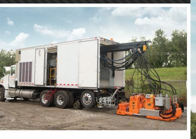
Progress Rail's Welding Division is a market leader in welding programs and equipment to improve weld performance and quality. Working with our international affiliate EO Paton, Progress Rail has developed a narrow head welder for our mobile units. This head can be used with our extended boom trucks when welding turnouts and in tight confines.
