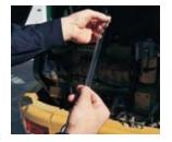
not have a dipstick, cut the tubing so that it reaches about halfway into the fluid depth.
