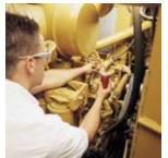
Coolant compartments with sampling valves can be sampled using the same steps as the oil sampling valve method described earlier.
