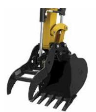
Cat thumbs work with buckets to grab, pick or sort material. They are hydraulically controlled from the cab, opening and closing around loads. And when you don't need it, the thumb can retract against the machine stick.
