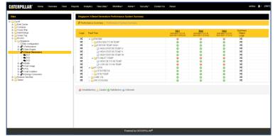
Performance summary view shows graphical health status of onboard equipment with sub-system breakdown. Asset tree on the left enables navigation between different systems. All of the analysis is based on qualified data.
