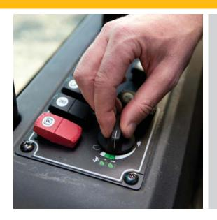
Eco Modes achieve significant fuel consumption reduction by allowing the engine to run at lower speed whenever possible, and rapidly increasing speed when power is needed. Designed to save fuel in light or medium duty applications, the extremely fast engine response allows these modes to be used even in power demanding applications and eliminates the need to constantly shift into and out of Eco Modes.
