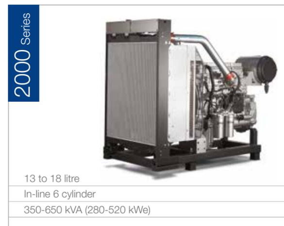
**Overview:** Developed from a proven heavy-duty industrial engine, the 2000 Series turbocharged chargecooled engines offer exceptional performance and fuel consumption in an ultra-compact package.
