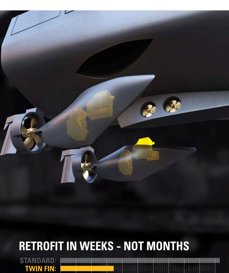
If your vessel is currently fitted with azimuth thrusters, retrofitting the twin fin propulsion system couldn't be simpler or quicker. The system is pre-fabricated so the work and downtime at the shipyard is reduced to a bare minimum – possibly even as little as a third of the time of a standard refit! After all, every hour is important.
