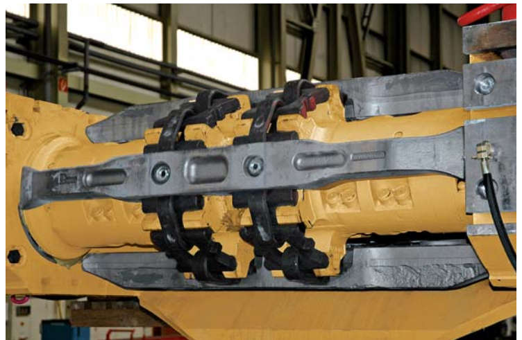
PowerChain and sprocket in use with a Cat beam stageloader
