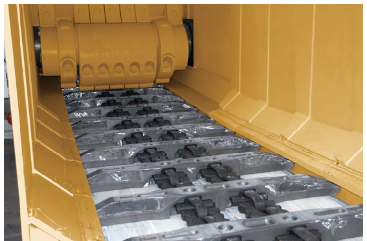
PowerChain inside a Cat BSL in the crusher area
