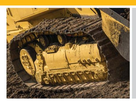
An oscillating undercarriage decreases ground shock to the machine, giving you increased stability and a smoother ride. Choose Sealed and Lubricated Track undercarriage for aggressive applications like land clearing, side-slopes or rocky terrain. Or, choose SystemOne™ undercarriage that is designed to work and wear as a system for longer life and lower costs in many applications. A choice of track shoe designs and widths help you further optimize your machine for performance and longer life.
