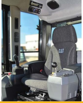
Updated cab gives operators added comforts like adjustable armrests and controls, improved air conditioning system and a heated/ventilated seat option. A new LCD operator interface makes it simple to customize machine performance features and to view machine operating and service information.
