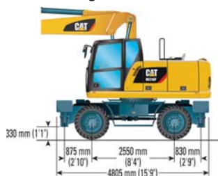
Undercarriage with 2 sets of outriggers
