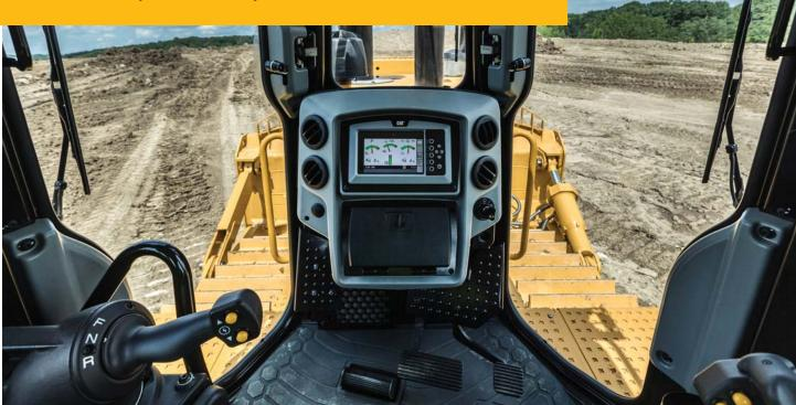
A quiet, comfortable cab, with an Integrated Roll Over Protection Structure (ROPS), gives operators greater all around visibility to enhance safety and productivity. Pressurization helps keep dust out for a cleaner operating environment. A low-effort single tiller-style handle controls direction and gear selection for ease of operation.
