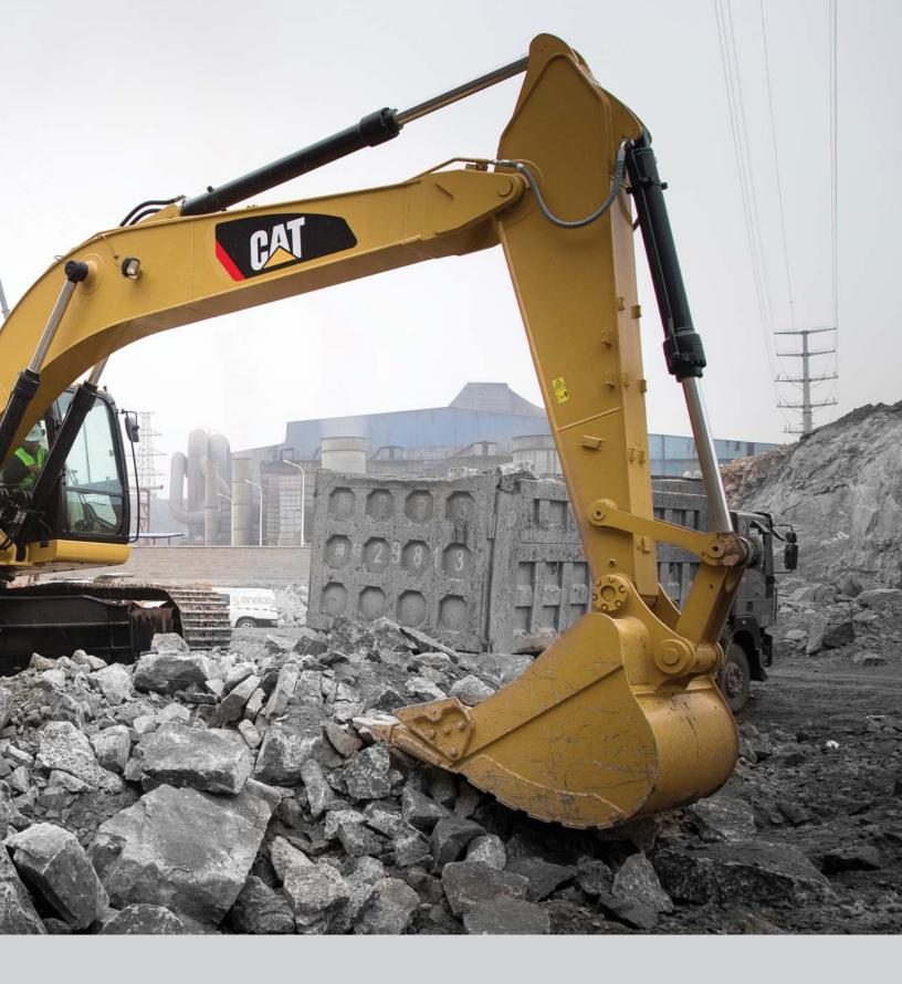
The 330D2 L comes with a number of new developments and features, including engine speed control, a new fuel filtration system, and a built-in economy mode to help decrease fuel consumption up to 15% (as compared to 329D L China Nonroad Stage II equivalent). A variable-speed fan with viscous clutch reduces noise and saves energy.
