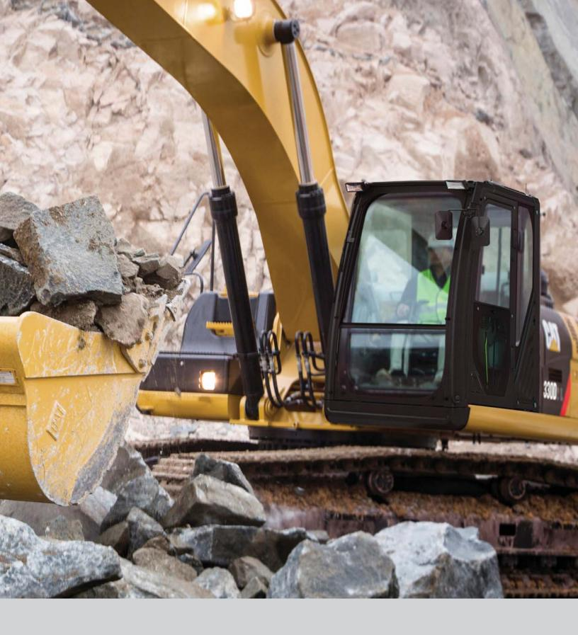
The 330D2 L comes with a number of new developments and features, including engine speed control, a new fuel filtration system, and a built-in economy mode to help decrease fuel consumption up to 15% (as compared to 329D L Tier 2/Stage II equivalent). A variable-speed fan with viscous clutch reduces noise and saves energy.
