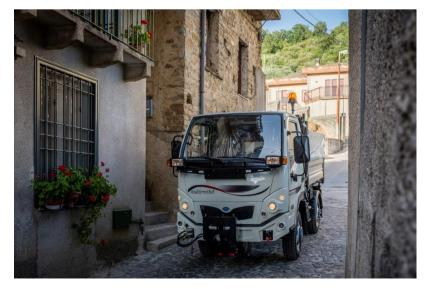
This year Durso presented a new model, with an even more compact size. Powered by the Perkins 404D-22T, which delivers the same power and higher torque, the engine was perfectly in line with the main concept of the MULTIMOBIL project to increase performance without added cost and complexity.
