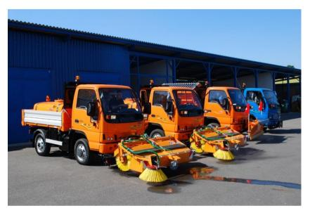
To meet these needs, Durso developed a completely new concept in multi-functional vehicles, that it says balances the relationship between cost and performance, thanks to its reliability and the possibility to install more than one PTO for the hydraulic system, plus the fact it uses a Perkins 404D-22 engine.
