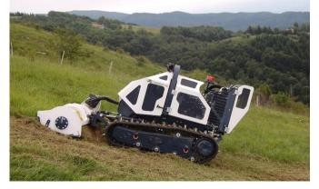
operator can see the working area. The rollover protection is also used to lift the machine.
