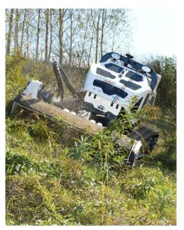
The self-tensioning and self-adjusting crawler makes sure the Herb-Hy doesn't compact the soil and works properly on every surface. On extreme slopes the machine keeps a straight path thanks to a hydraulic offset regulator on a hydraulic motors circuit. The crawl track can be adjusted between 1.3 and 1.8 meters.
