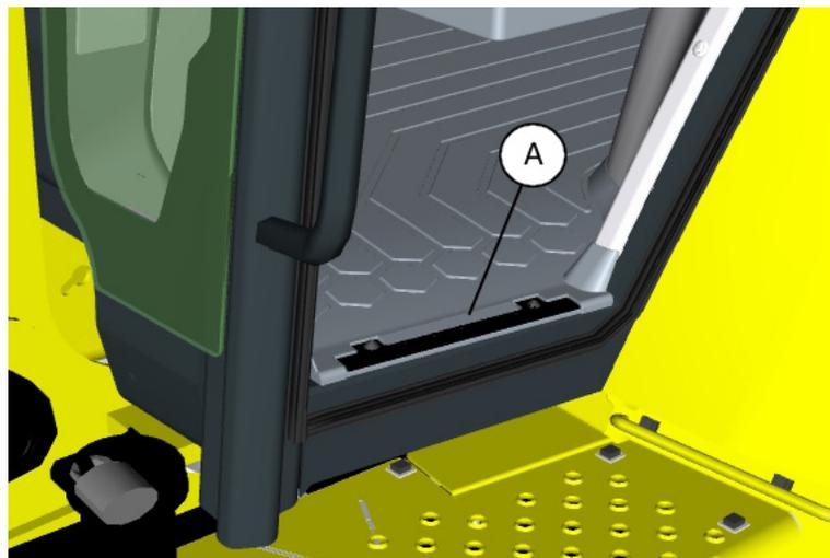
3. Remove door treads (A) and roll back the front part of the floor mat.
