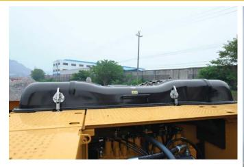
**Anti-skid plating** covers the entire upper structure and storage box to prevent slipping during maintenance. Safety is further enhanced with the addition of countersunk bolts to reduce trip hazards.
