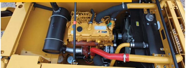
The Cat C4.4 ACERT engine with four cylinders has been designed to meet U.S. EPA Tier 3/EU Stage IIIA equivalent and China Nonroad Stage III emission standards. The proven C4.4 ACERT engine incorporates robust components and precision manufacturing you can count on for reliable and efficient operation. Less sensitive to low quality fuel, it boasts improved reliability while delivering reduced fuel consumption.
