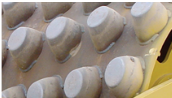
Oval pads are a good match for cohesive soils and thicker lifts.
