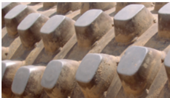
Square pads are best suited for semi-cohesive soils and thinner lifts.
