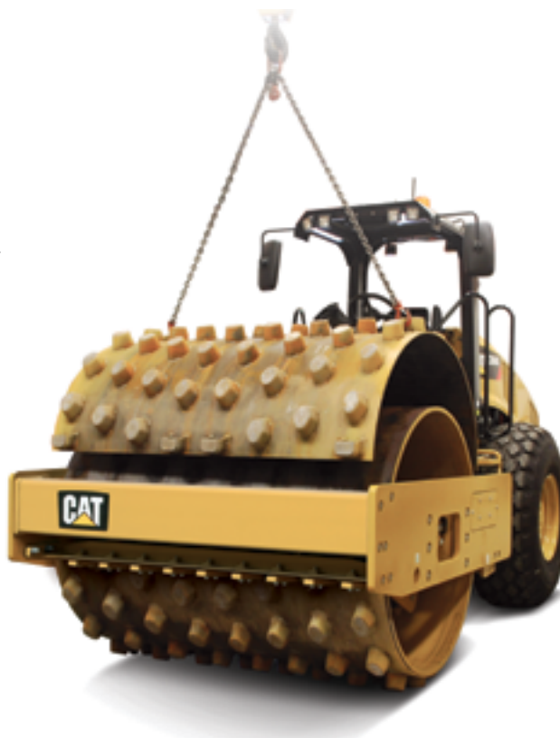
Caterpillar also offers a padfoot shell kit option for smooth drum compactors. The two-piece shell bolts onto the smooth drum, allowing the compactor to be used on cohesive soils like a normal padfoot drum. Both square pad and oval pad shell kits are available.
