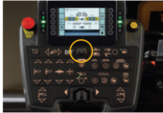
Mix height dials at the screed control panels regulate the head of material at the ends of the auger shafts.
