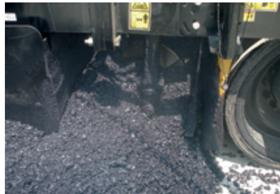
Mechanical feeder sensors contact the material as it flows out of the auger chamber.
