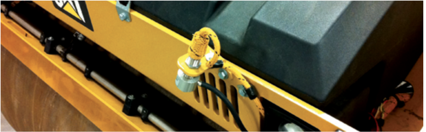
Infrared sensors send temperature data to the display in the operator’s compartment.
