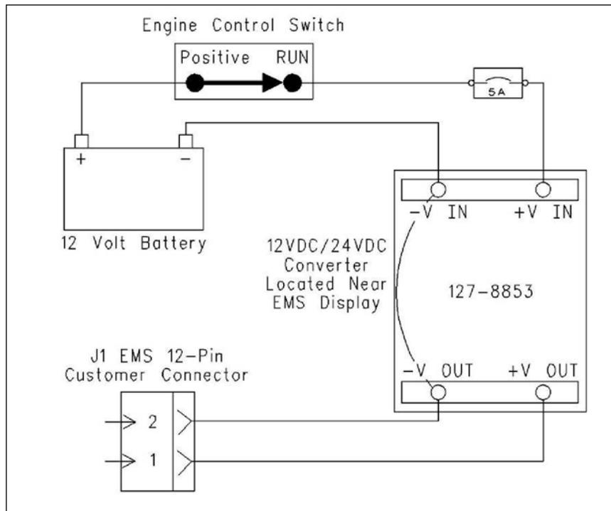
**Figure 7-9 12 Volt Battery Connections w/Converter**
