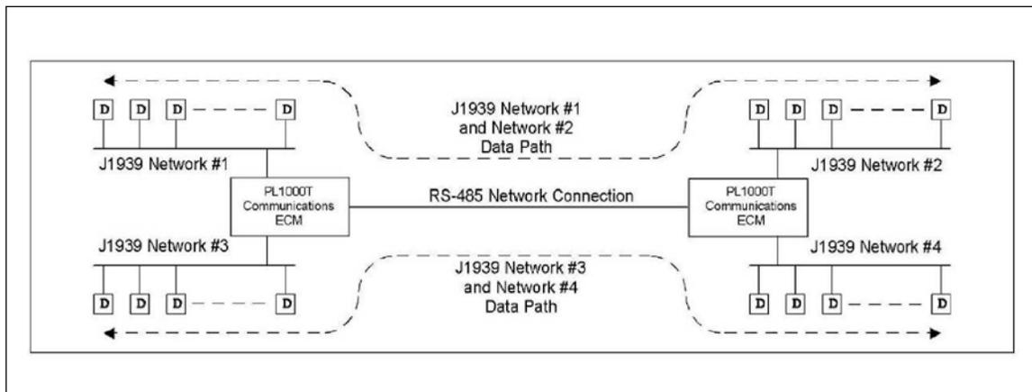
**Figure 12-11 PL1000T Configured for the CAN Extension Bridge Network**
