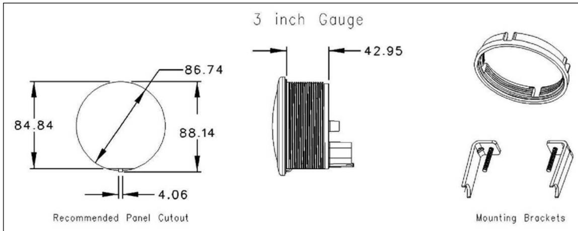
**Figure 6-4 Mounting Dimensions for 76 mm (3.0 Inch) Gauges**
