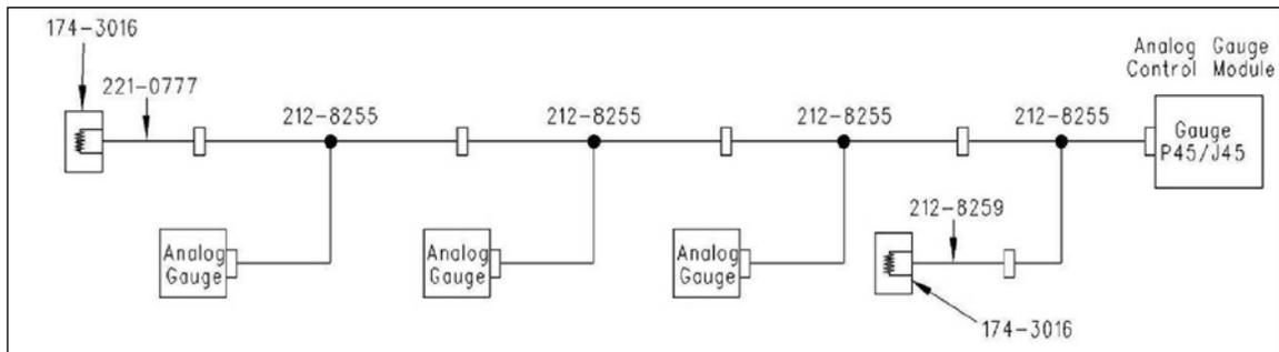
**Figure 6-6 Diagram for Analog Gauges**
