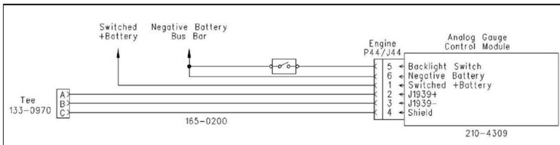
**Figure 6-5 Drawing for Connecting the Analog Gauges to the J1939 Data Link**
