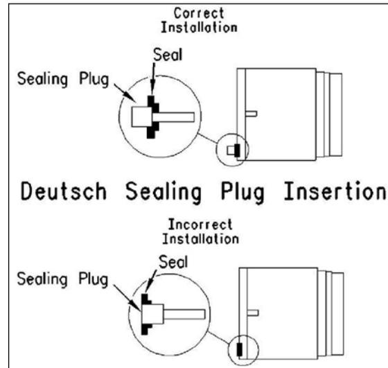
**Figure 3-2 Installation of Seal Plugs**
