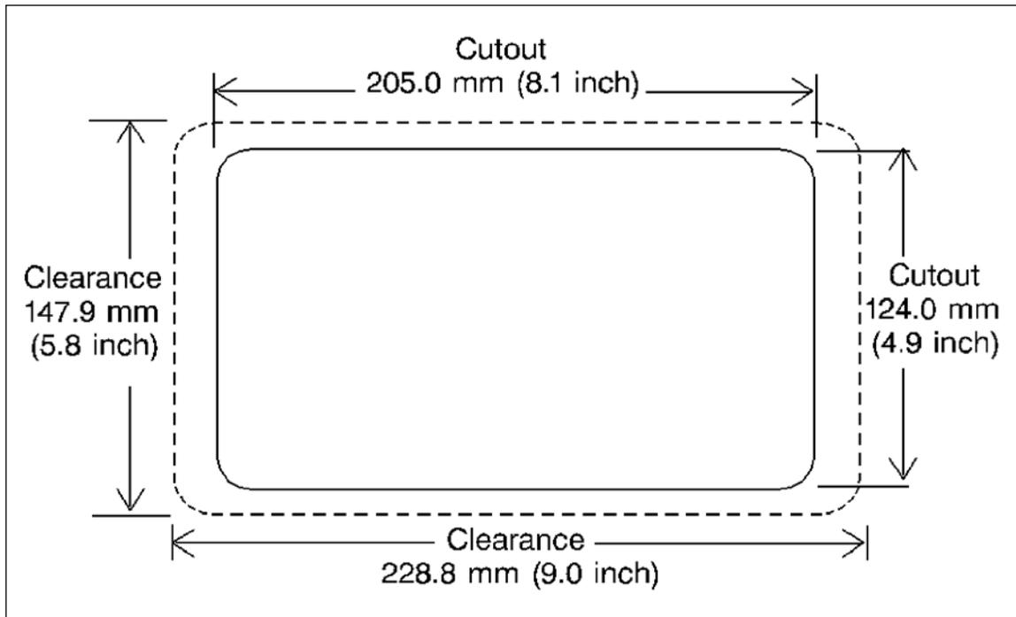
Figure 10-8 Marine Power Display (Cutout not to scale)
