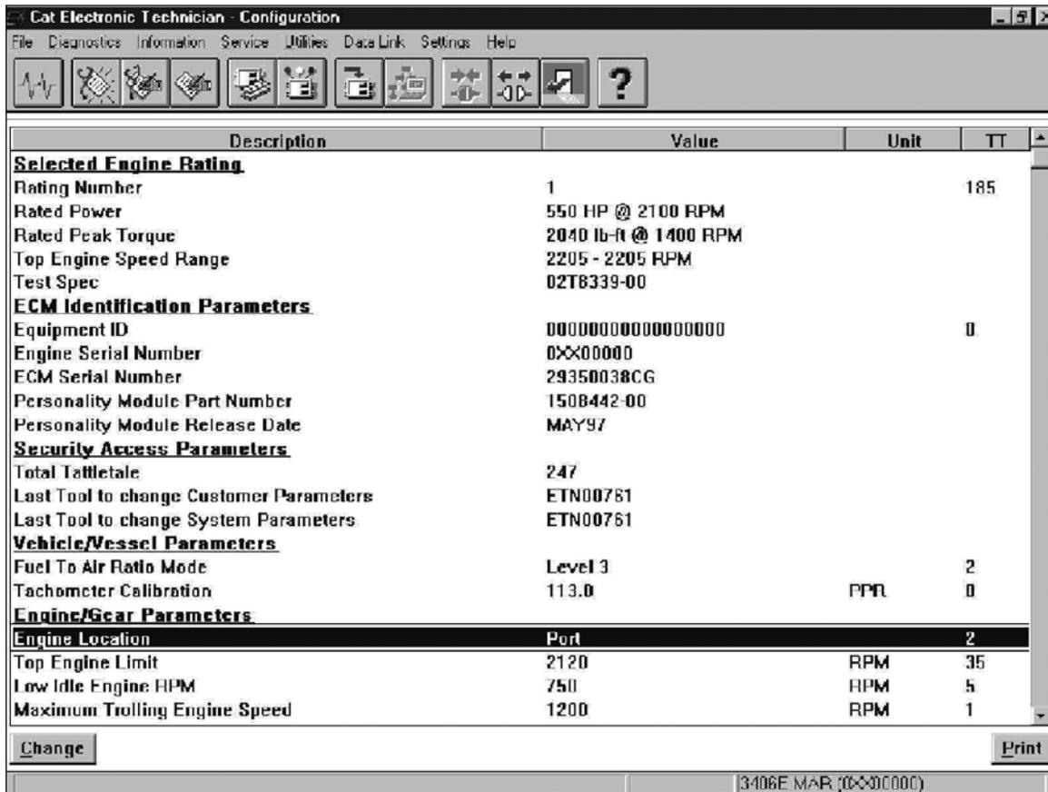
Figure 8-3 Selecting Engine Location
