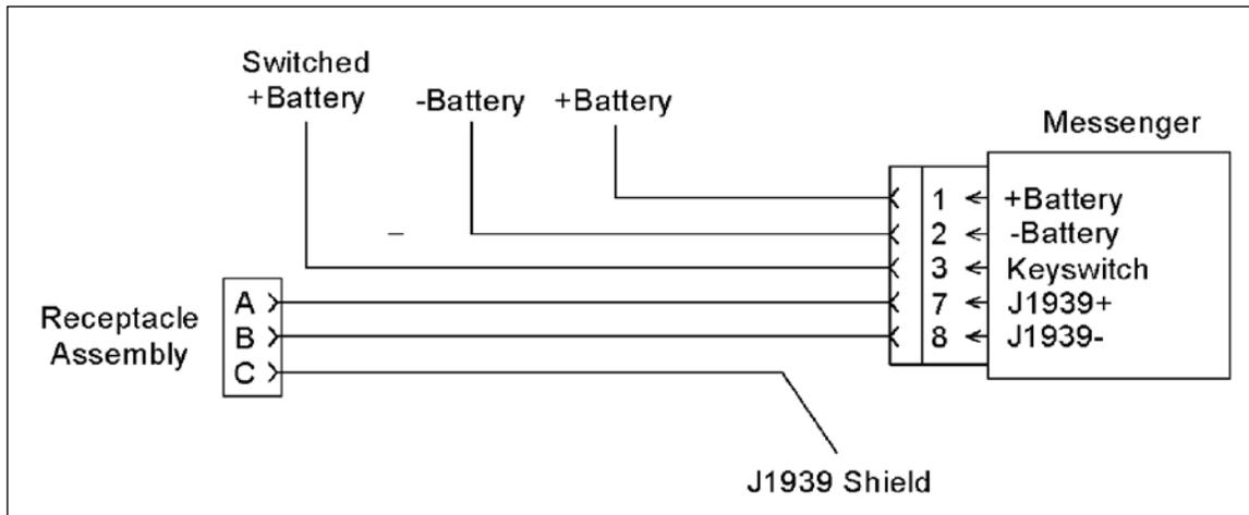
**Figure 11-6 Messenger Wiring Diagram**
