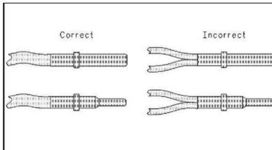
**Figure 3-1 Terminal Connections**
