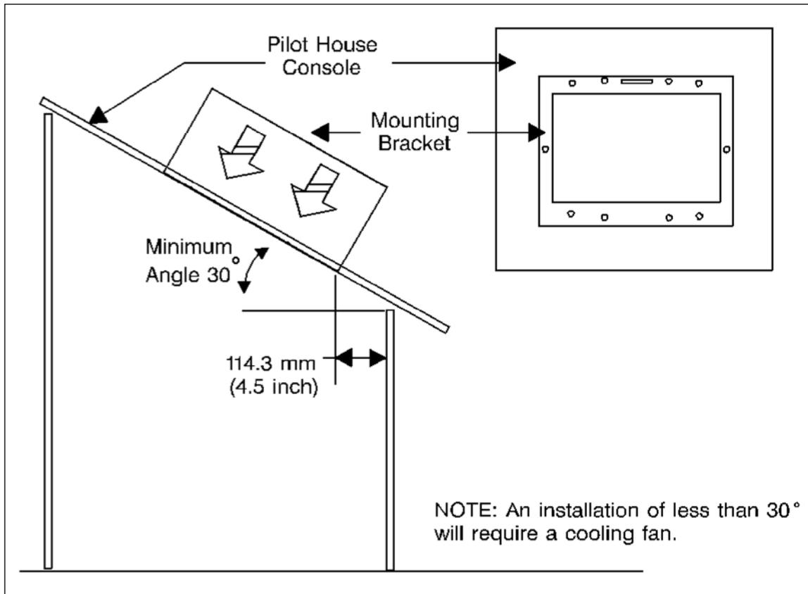
**Figure 8-7 Mounting Location**
