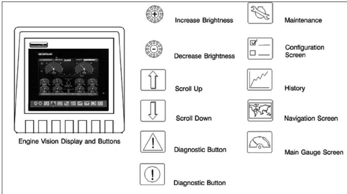
Figure 8-2 Controls for the Engine Vision
