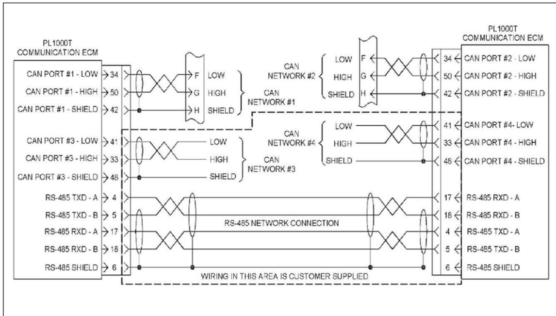
**Figure 12-12 PL1000T Communication ECM Configured As a CAN Extension Bridge Network**
