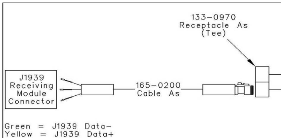
**Figure 5-8 Connecting a J1939 Module**
