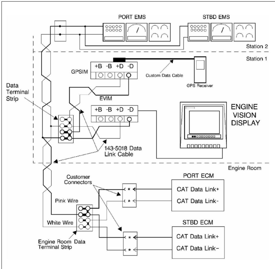
**Figure 8-18 EVD Connections to Cat Data Link**
