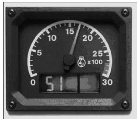
**Figure 7-3 Tachometer Gauge Module**
