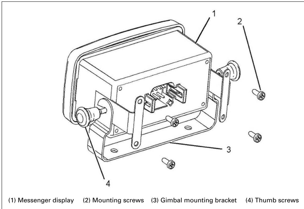
**Figure 11-7 Messenger Display Rear View**
