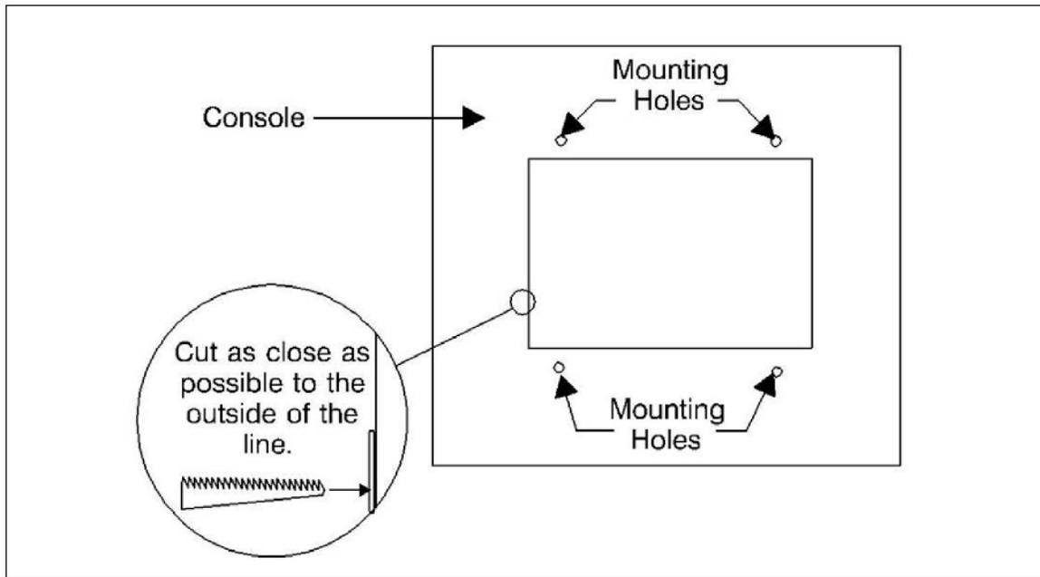
**Figure 8-9 Cut the Console**
