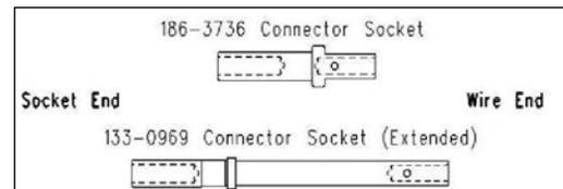
**Figure 5-6 Connector Sockets**
