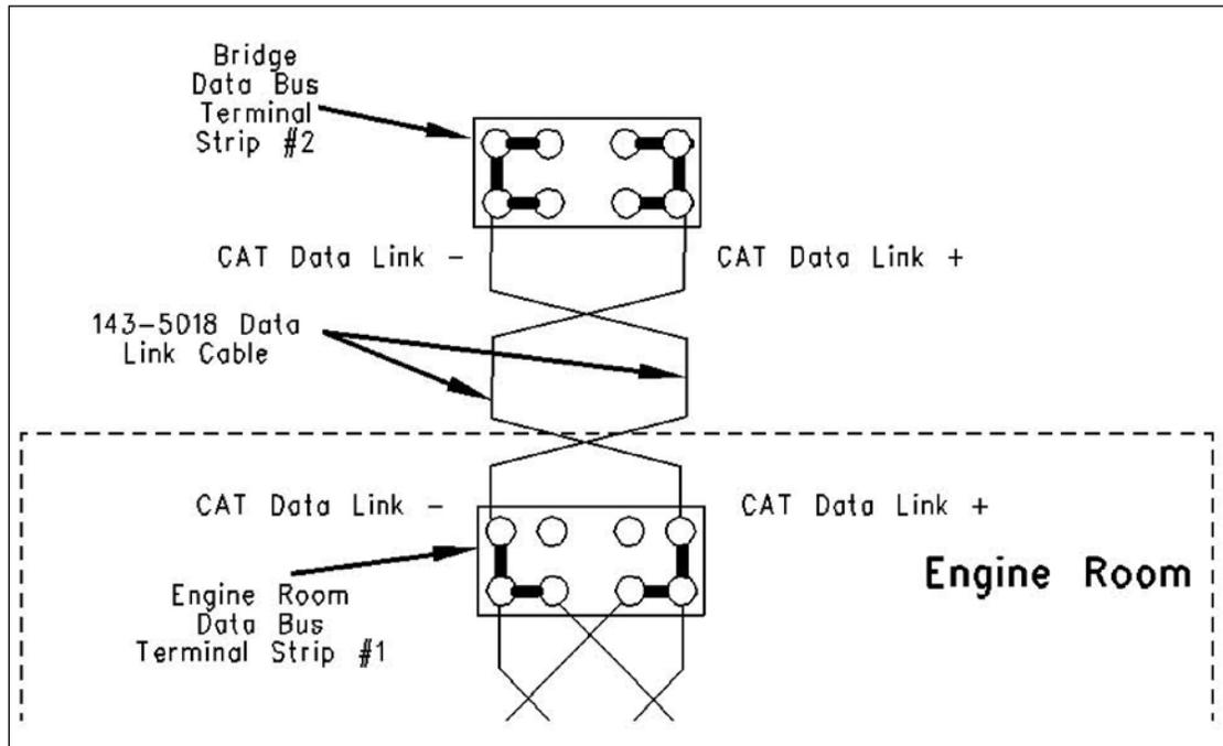
**Figure 5-2 Connections from the Engine Room to the Bridge**
