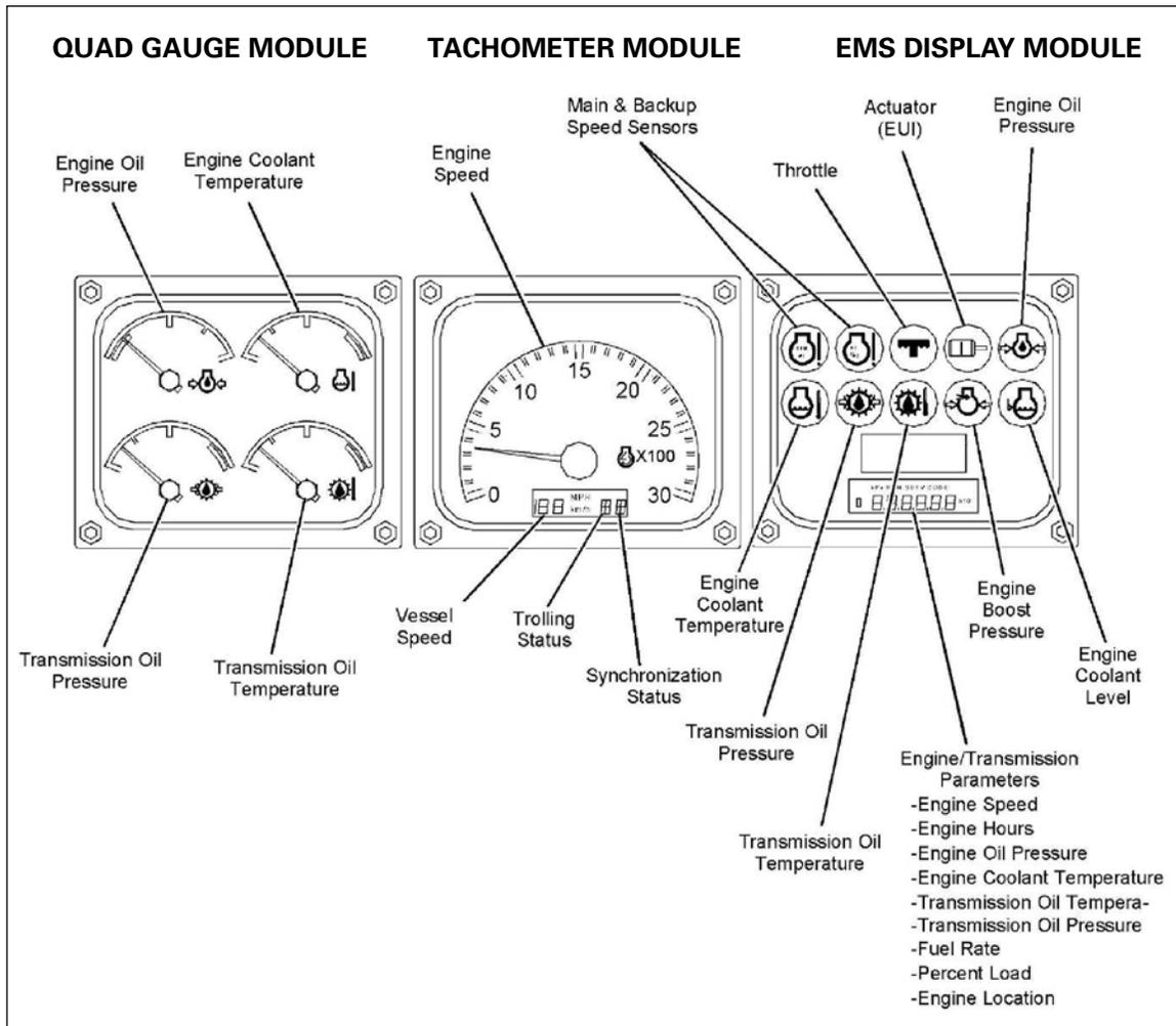
**Figure 7-5 Display for the Engine Monitoring System**
