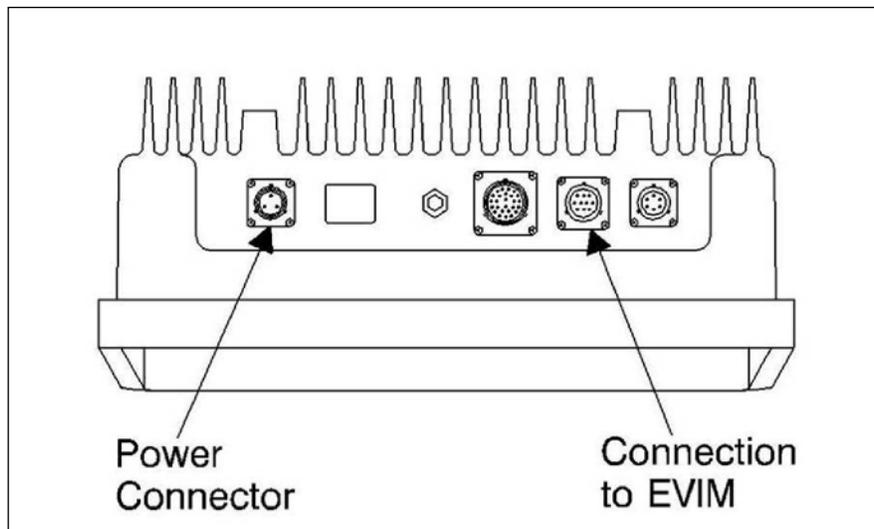
**Figure 8-17 Connections for the Engine Vision Display**
