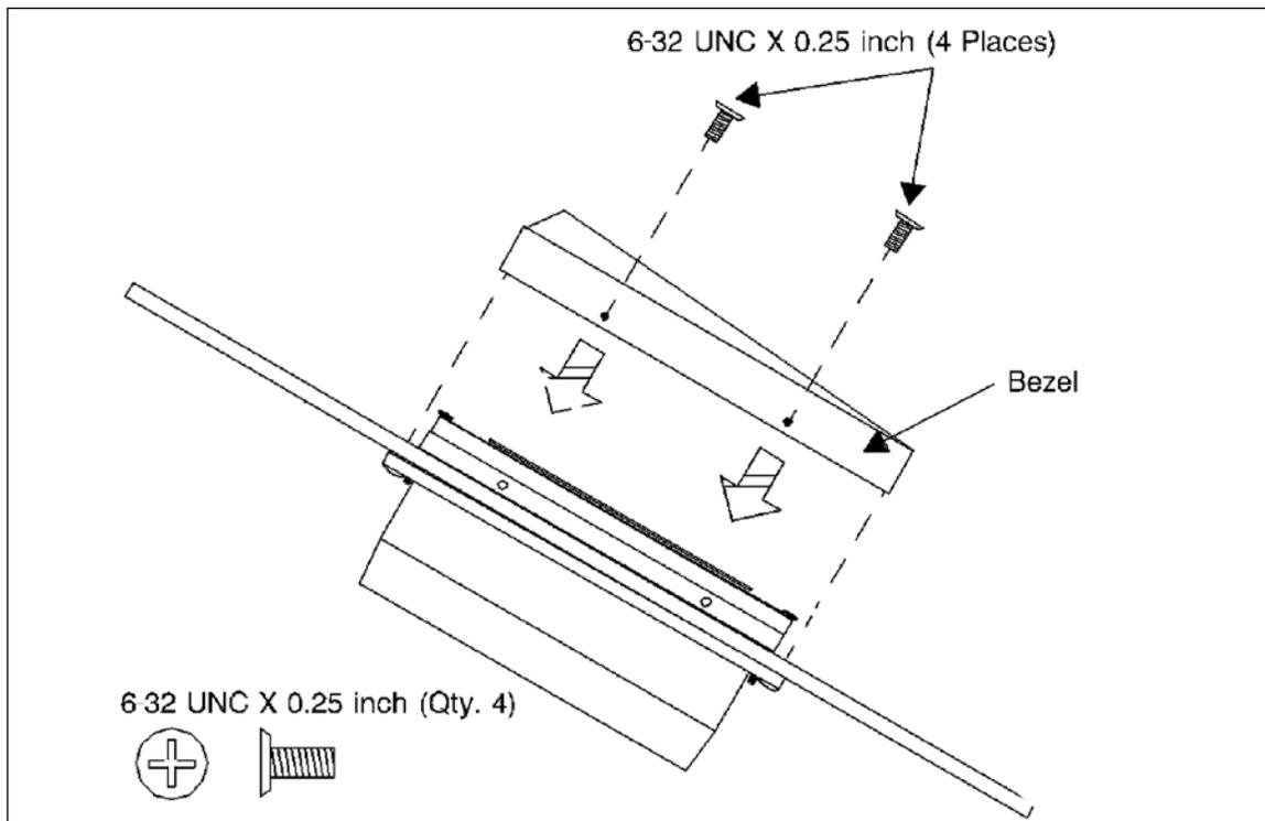
**Figure 8-14 Attach the Engine Vision Display**
