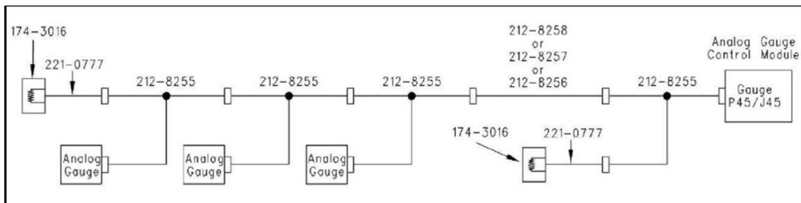
**Figure 6-7 Diagram for Analog Gauges w/Harness**
