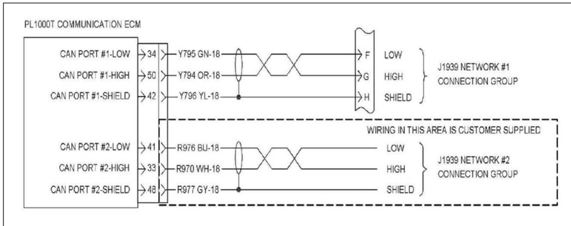
**Figure 12-8 J1939 Bridge Diagram**
