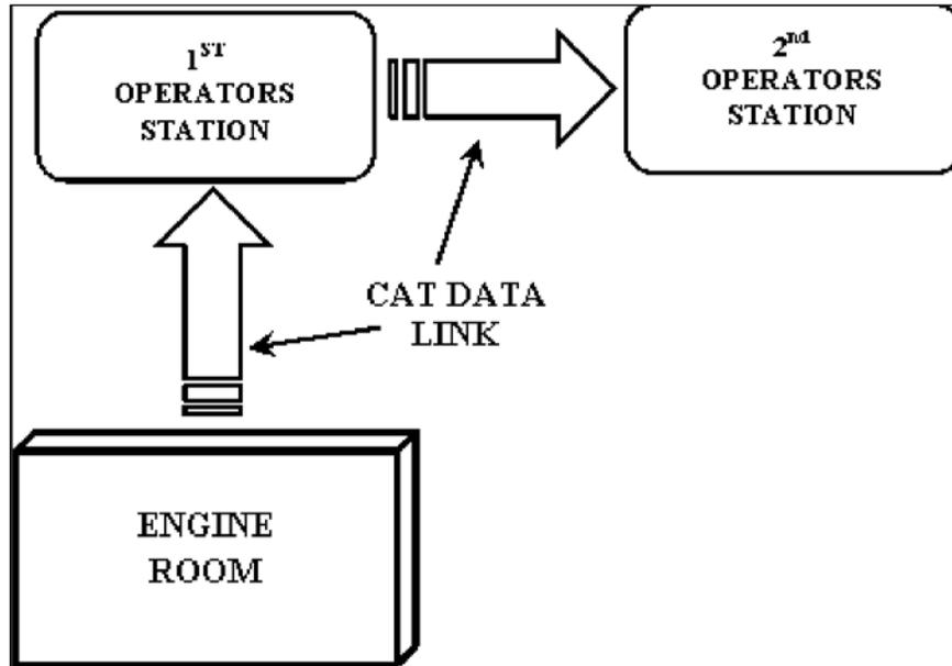
Figure 5-3 Second Operator Station
