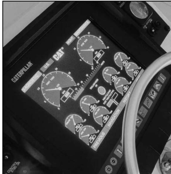
**Figure 8-1 Engine Vision Console**
