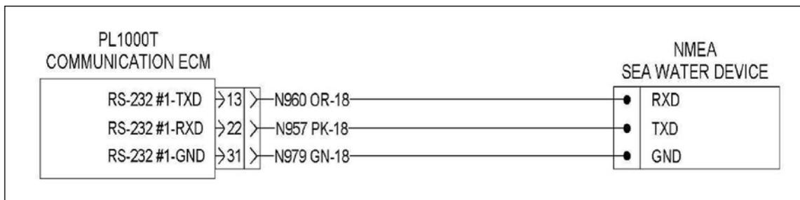
**Figure 12-2 RS232 PL1000T Connections To NMEA Sea Water Device**
