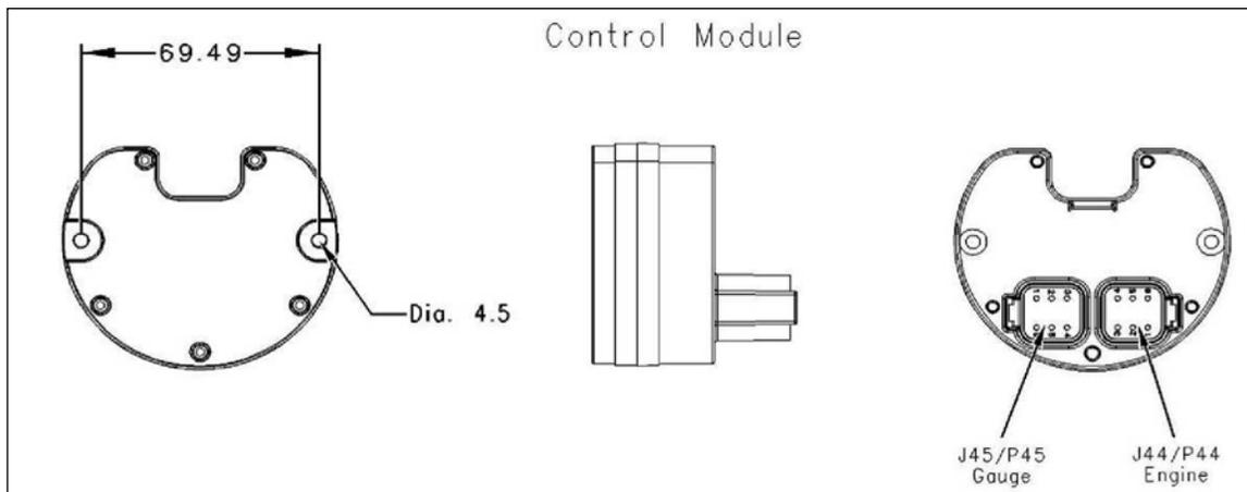
**Figure 6-2 Mounting Dimensions (mm) Control Module**
