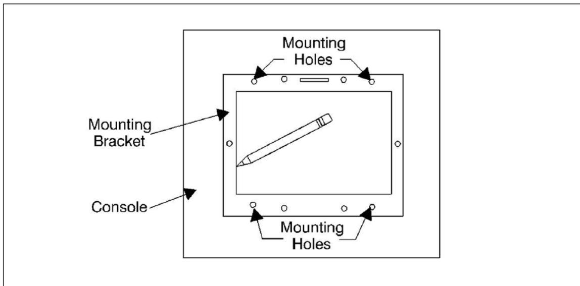
**Figure 8-8 Trace the Mounting Bracket**
