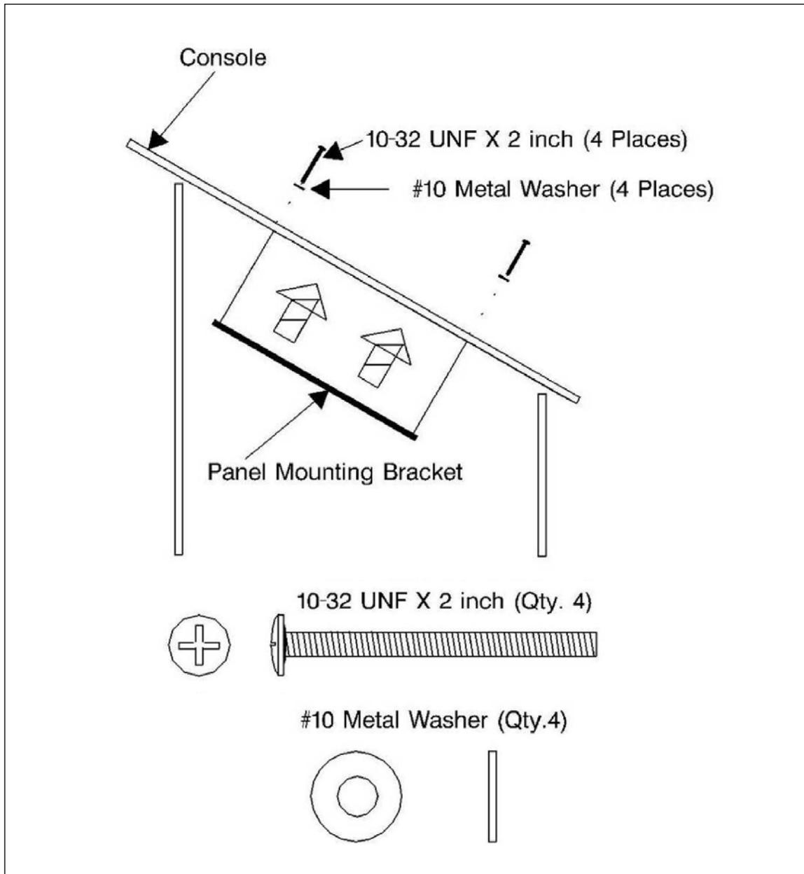
**Figure 8-10 Install the Mounting Bracket**
