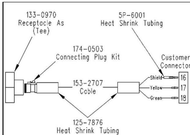
**Figure 5-5 Connecting Customer Connection to Tee**
