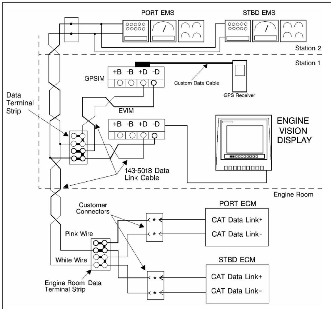
**Figure 9-3 Connections for the Cat Data Link**
