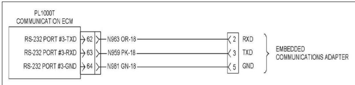
**Figure 12-15 Connections for Embedded Communications Adapter**
