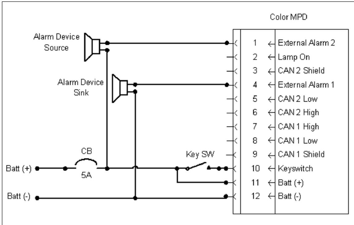
**Figure 10-19 Color MPD with Alarms 300 mA Current or Less**
