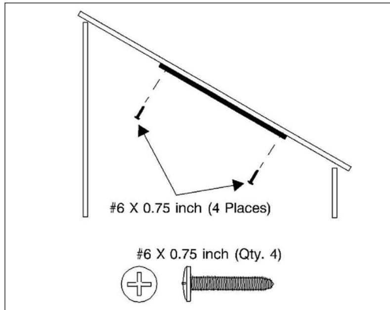
**Figure 8-11 Secure the Mounting Bracket**
