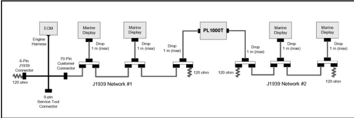
Figure 12-17 PL1000T CAN Extension Example
