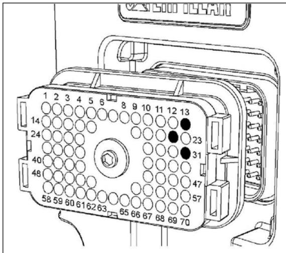
**Figure 12-3 70-Pin Connector —
