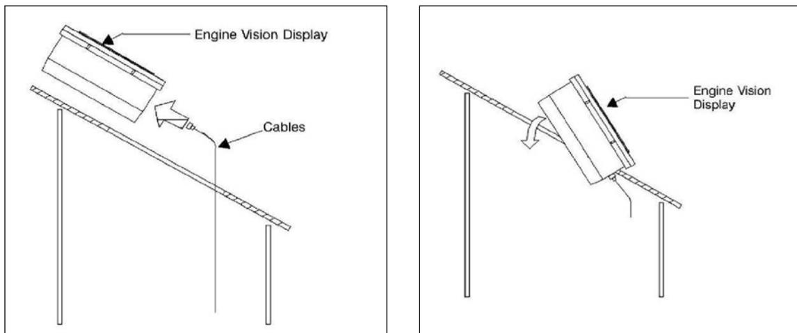
**Figure 8-12 Install the Engine Vision Display**
