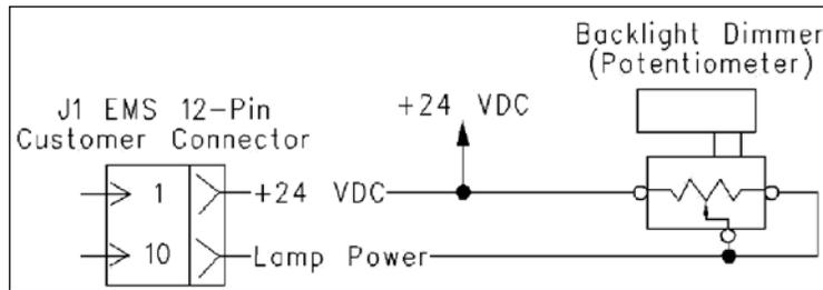
**Figure 7-17 Drawing For the Potentiometer**
