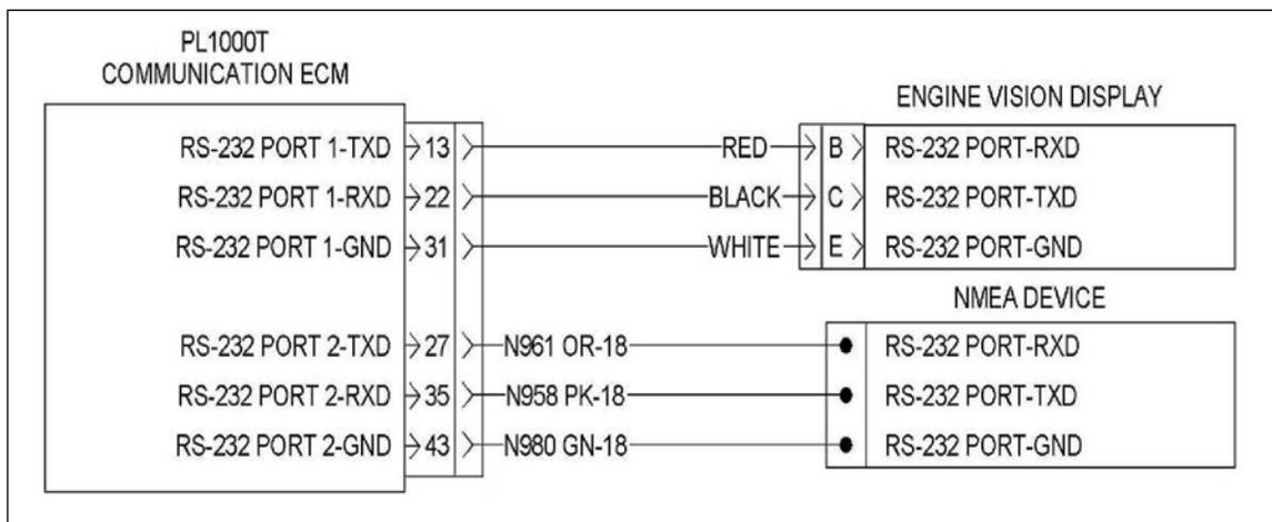
**Figure 12-4 RS-232 to Engine Vision**
