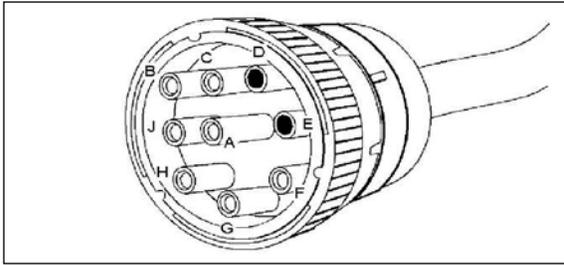
**Figure 12-14 9-Pin Connector**
