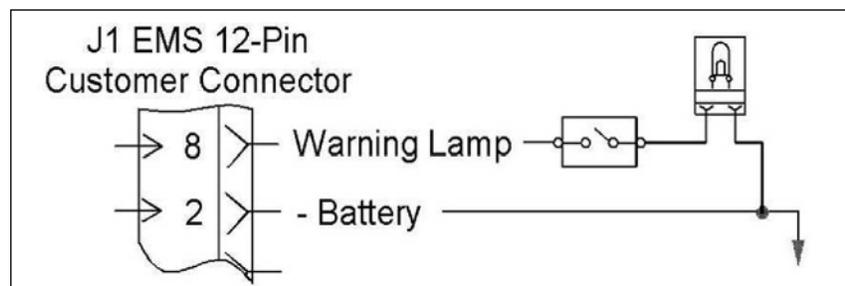
**Figure 7-15 Warning Lamp****Table 7-9 Warning Lamp Required Parts**
