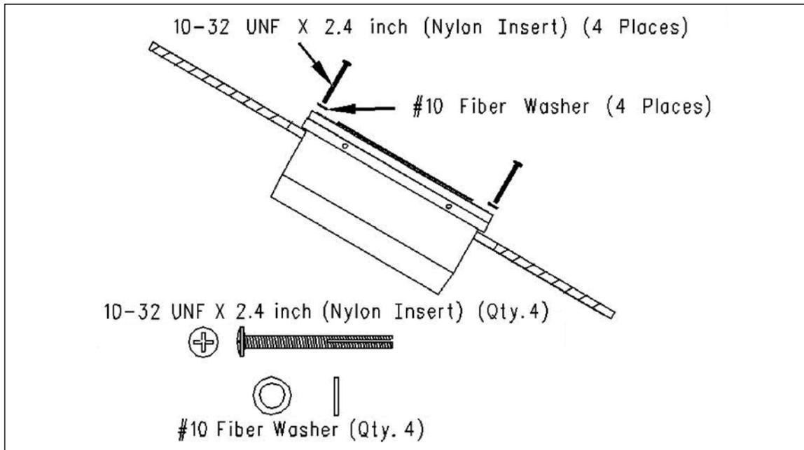
**Figure 8-13 Secure the Engine Vision Display**
