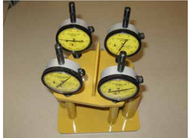
Figure 6: New Valve Recession Measurement Tool for Cat® G3500C/E Engines
