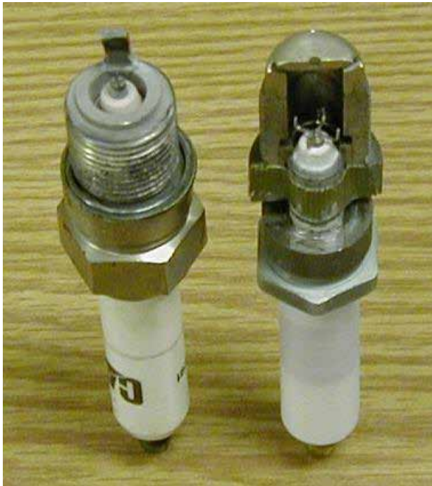
Figure 4: J-Gap (left) Versus Prechamber (right) Spark Plugs
