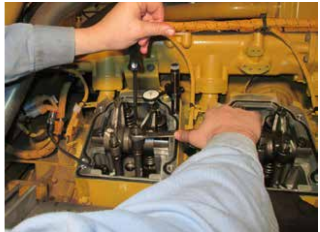
Figure 7: Valve Lash Adjustment
