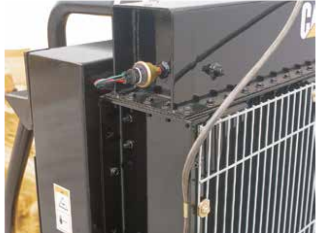
Figure 8: Coolant Level Sensor in a Cat® G3406 Engine
