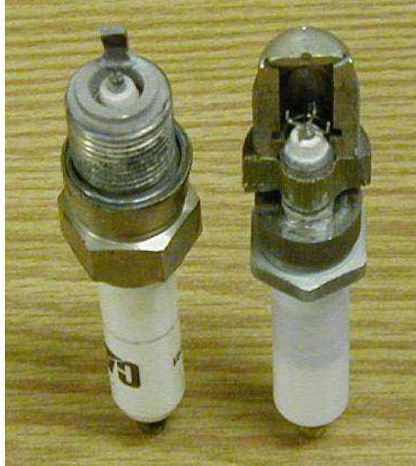
Figure 4: J-gap (left) and prechamber (right) spark plugs
