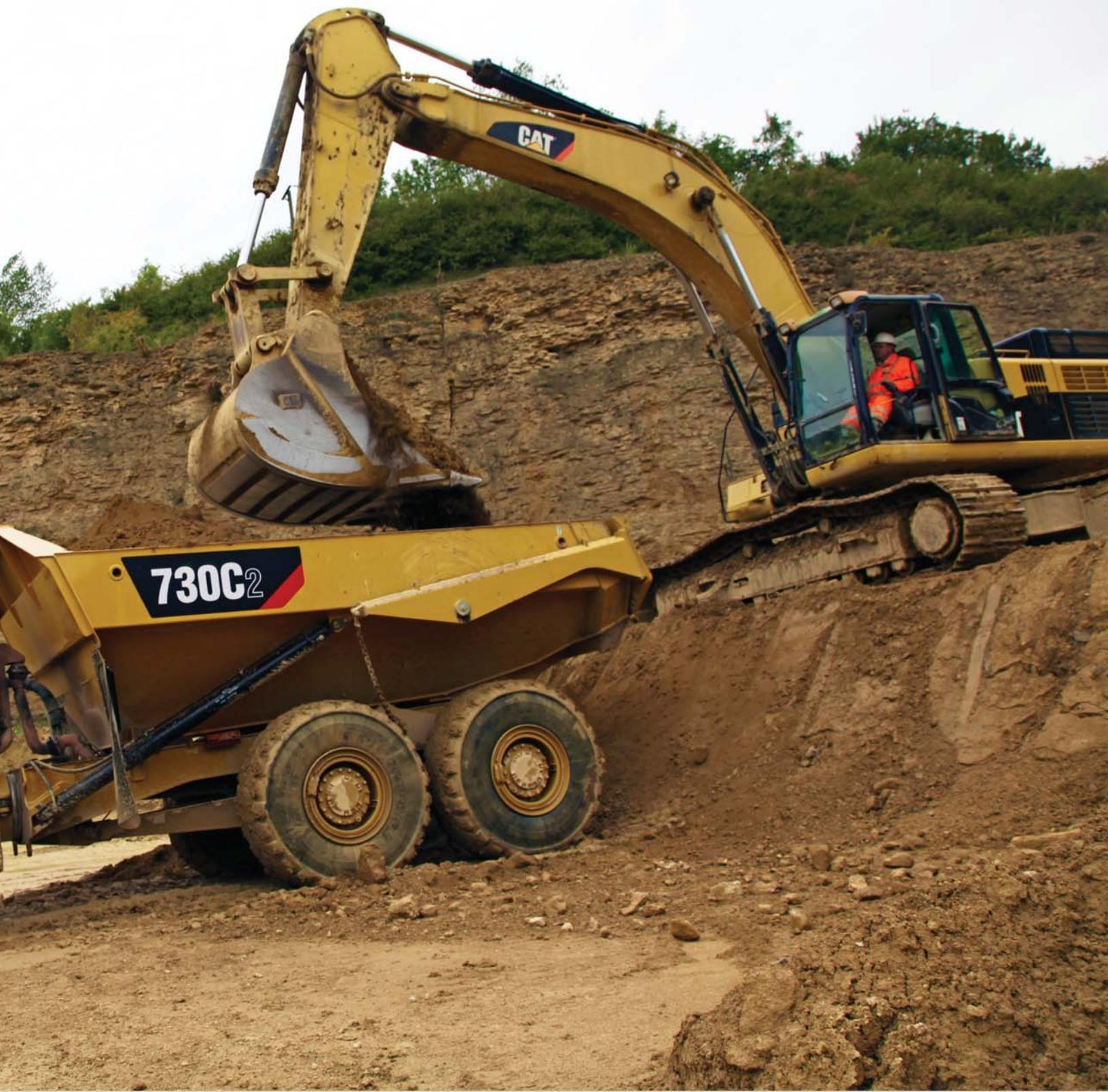
The Cat 730C2, with a 17 m<sup>3</sup> (23 yd<sup>3</sup>) 28 tonnes (31 tons) capacity, offers demonstrated reliability and durability, high performance and productivity, superior operator comfort and lower operating costs.
