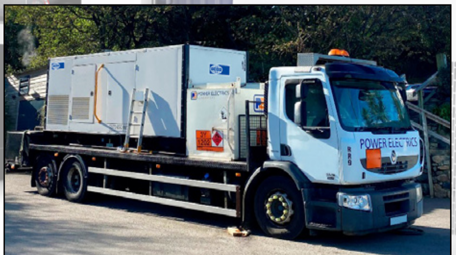
Rapid Response vehicle set up for rapid response designed to get to sites quickly and do not require unloading to supply power.
