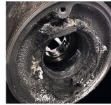
The risk of oil leakage past the piston ring seal is increased, particularly at the turbine end.
