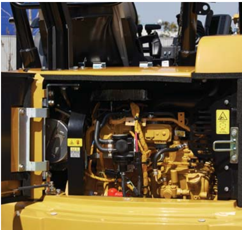
2) Engine service door to the concentrated service points
