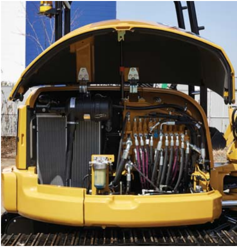
1) Side cover provides wider opening
