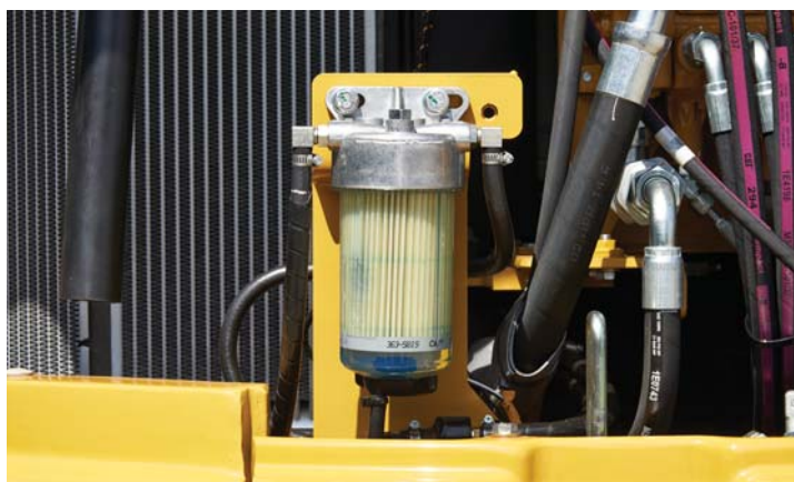
5) Water separator shaped fuel filter
