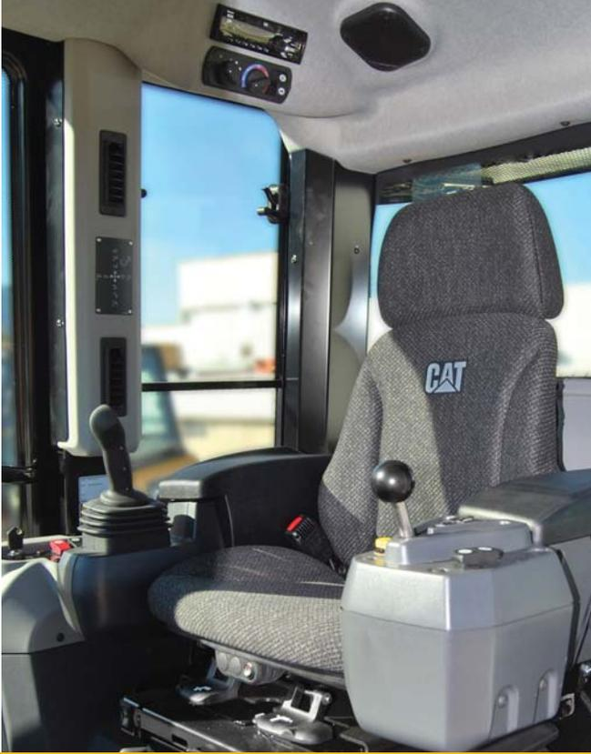
Updated cab gives operators added comforts like adjustable armrests and controls, improved air conditioning system and a heated/ventilated seat option. A new LCD operator interface makes it simple to customize machine performance features and to view machine operating and service information.
