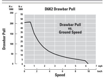
• The direct injection electronic fuel system provides a controlled fuel delivery increase as the engine lugs back from rated speed. This results in increased horsepower below rated power. A combination of increased torque rise and maximum horsepower improves response, provides greater drawbar pull and faster dozing cycles.
