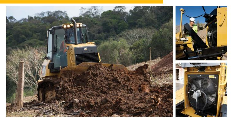
The engine radiator, Air To Air After Cooler (ATAAC), and hydraulic oil cooler are packaged in a single plane. Aluminum bar plate construction provides durability and allows for higher heat transfer and superior corrosion resistance.
