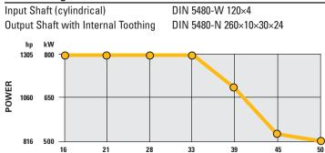
GEARBOX RATIO i [-] Rated Power P [hp] @ 60 Hz Rated Power P [kW] @ 50 Hz
