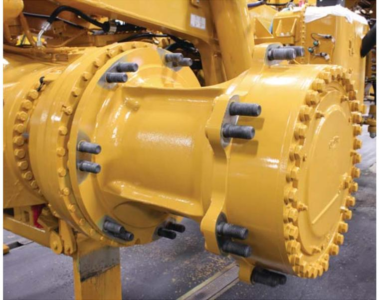
Extending brake life can also be achieved by choosing the optional Cat Engine Brake. This Caterpillar design works in conjunction with the ARC to slow the machine.
