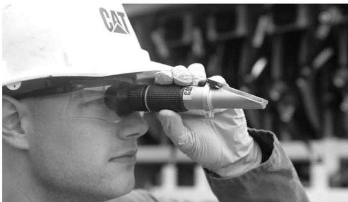
Too much or too little glycol will reduce the coolant's ability to provide protection to the cooling system. Heat transfer is affected by glycol concentration. Excessive levels of glycol will reduce heat transfer. Freezing Point and Boiling Point are calculated from Percent Glycol.
