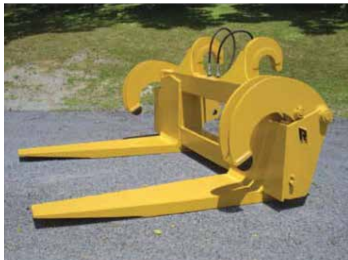
Pushbeam grapple equipped with coupler brackets
