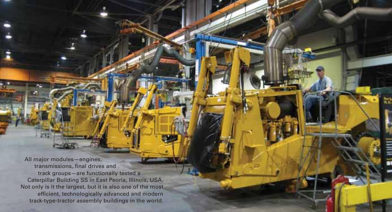
All major modules—engines, transmissions, final drives and track groups—are functionally tested at Caterpillar Building SS in East Peoria, Illinois, USA. Not only is it the largest, but it is also one of the most efficient, technologically advanced and modern track-type-tractor assembly buildings in the world.
