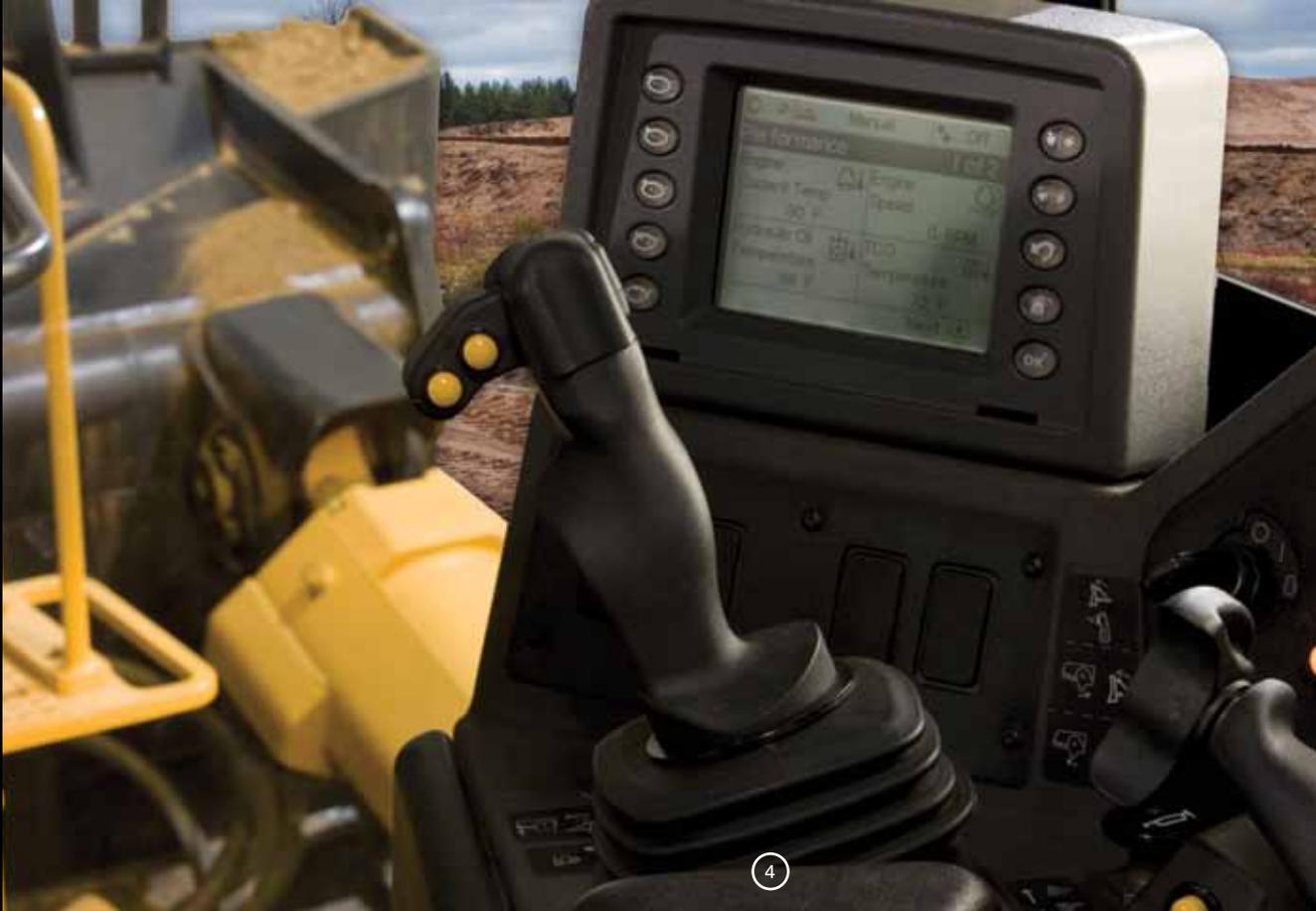
3. Visibility arrangements enhance visibility to the sides and rear of the machine. The Work Area Vision System (WAVS) camera system includes an adjustable LCD color monitor with auto-sense illumination for changing light conditions and a 115-degree panoramic viewing angle.
