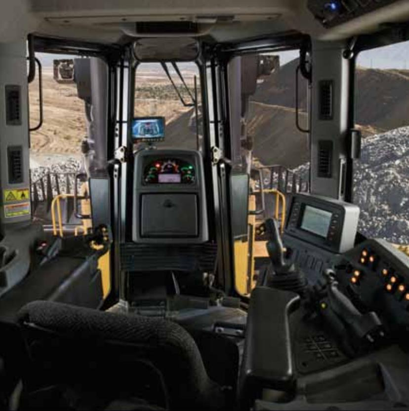
Cat® T Series tractors offer a new state-of-the-art cab that reduces operator fatigue for increased performance. With 30 percent more glass and a 15 percent wider cab, it's designed for operator comfort, convenience and productivity. Some of the new features include: single hand steering control, fully adjustable air suspension seat, adjustable armrests, and increased storage space. The cab is also isolation-mounted to reduce noise and vibration for the operator.
